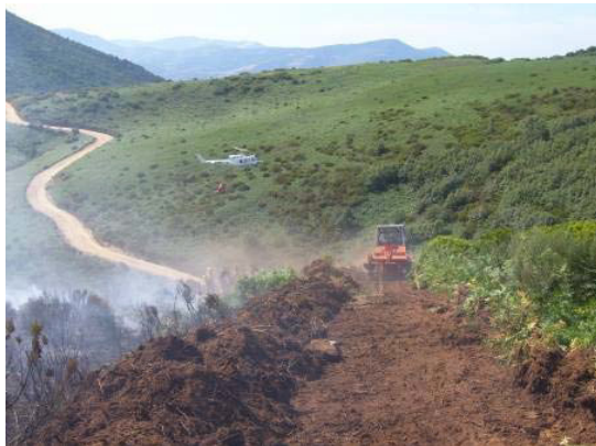
Figure 4 – Use of a Dozer for Fire Suppression
